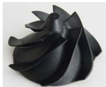
Impeller made using “XecoT”
